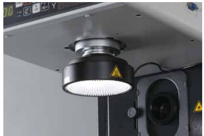
Example of attaching the LED circular illuminator to the PJ-PLUS
