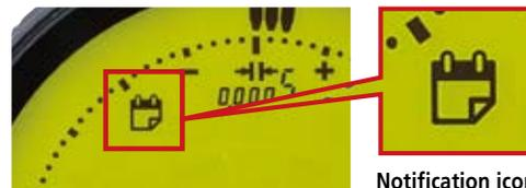
The calibration schedule warning icon starts blinking at a set time (e.g. 1 week before the calibration date) before the limit. If the limit is exceeded, the entire screen starts blinking to notify the user.
